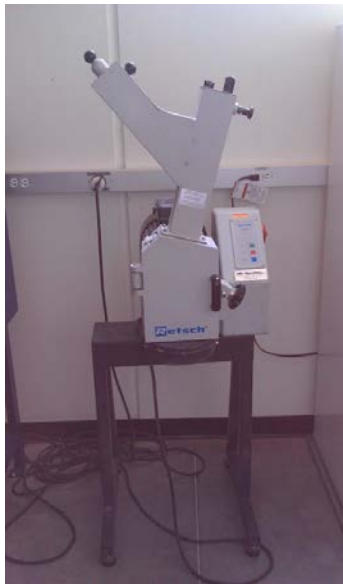
Knife Mill in Biomass Prep Room
