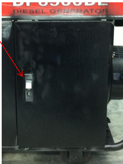
Figure 2- Press button identified by the arrow. Lift and pull lever to open the door.
