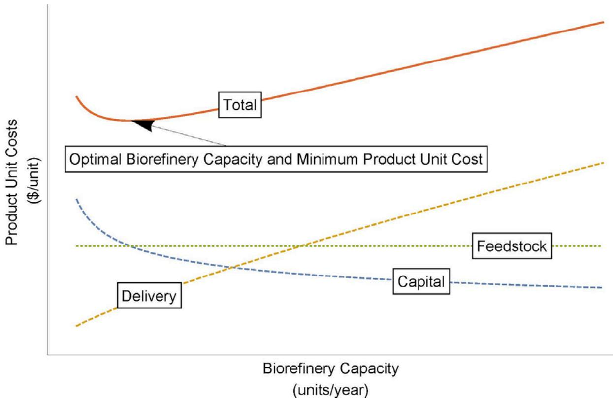
Figure 2: Trade-offs between increasing biomass delivery and decreasing biorefinery capital costs lead to a minimum total biofuel production cost based on capacity.
