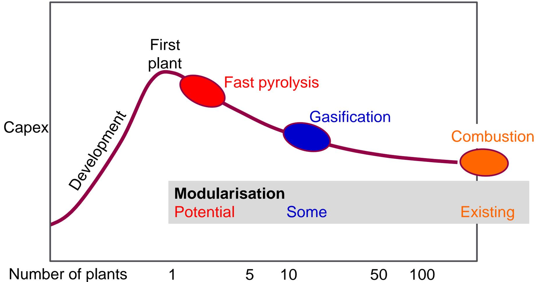
Modularisation depends on technology maturity, scale of process, and complexity of process
