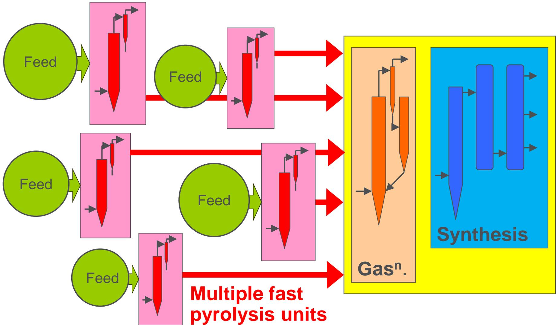
Higher cost for pyrolysis units, lower costs for gasification
