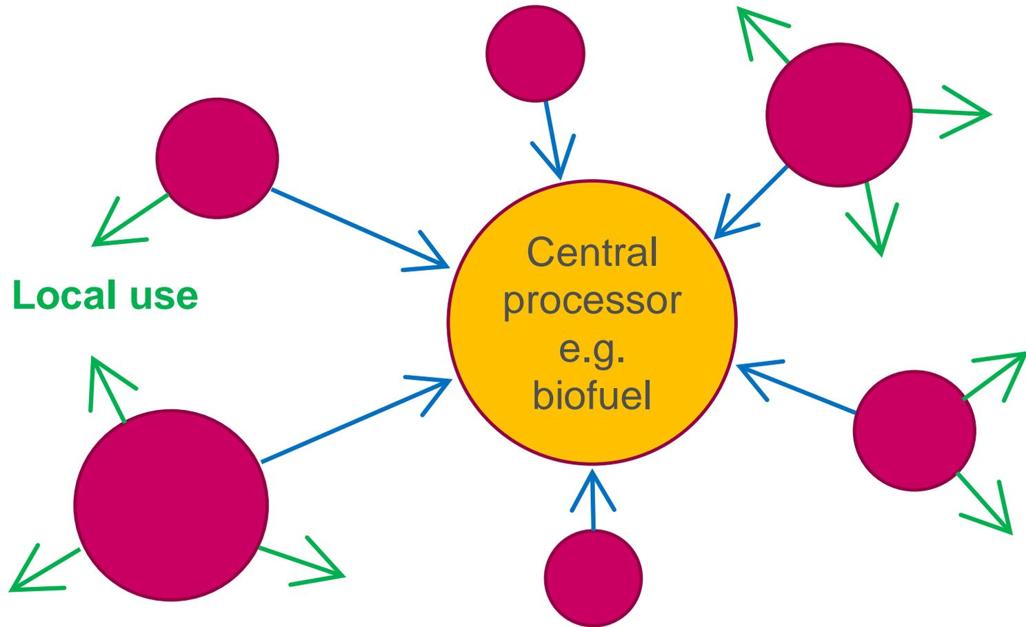
Decentralised fast pyrolysis systems could use modularisation when concepts and technology are better established
